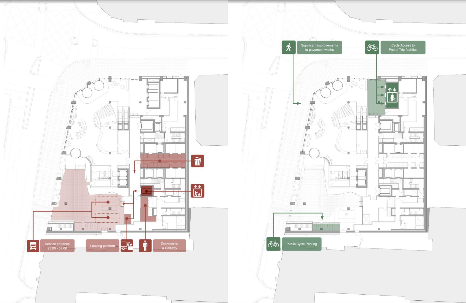
Ground Floor_Servicing & Cycle Access
